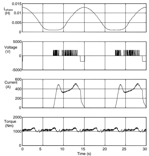
Figure 9: Half-voltage current-profiling (1000 rpm, 1000 Nm)
