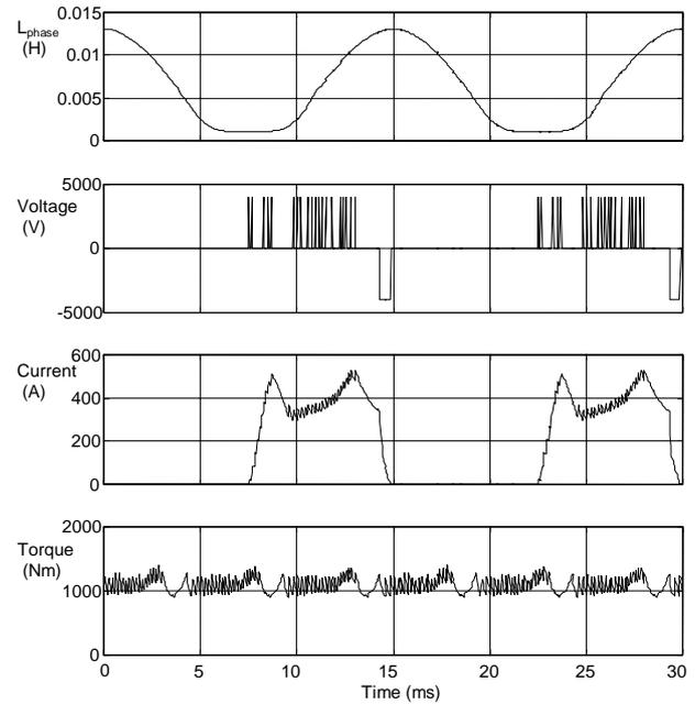
Figure 8: Full-voltage current-profiling (1000 rpm, 1000 Nm)
